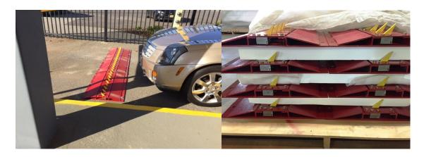
Carefully determine the location for your Directional Traffic Spike Control Units. Locate so that when the tires of the vehicle pass over the teeth they are parallel to the teeth. Place the units at least 15' - 20' into the lane.
